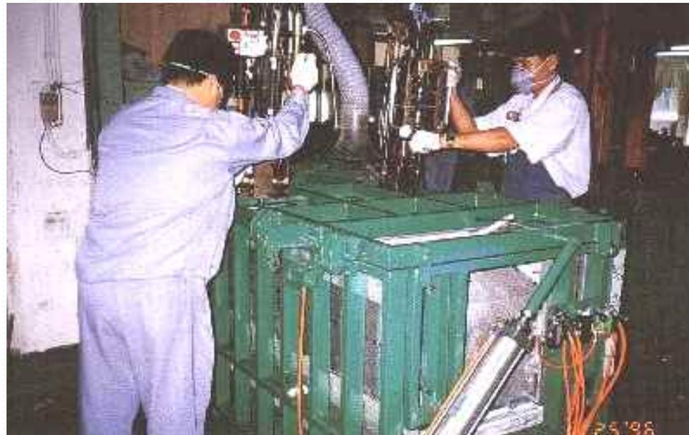
Figure 12 Even if isocyanate is used in an enclosed system, respiratory protection is still necessary
