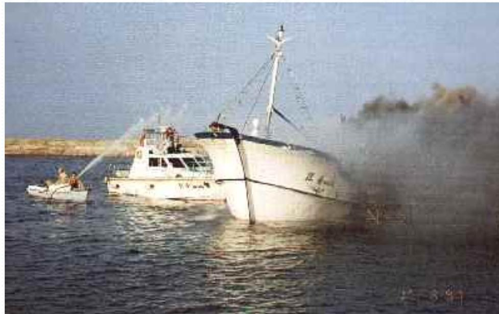
Figure 11 Fires often occur from the main motor in the center of the fishing boat because of carelessness during maintenance or mechanical failure
