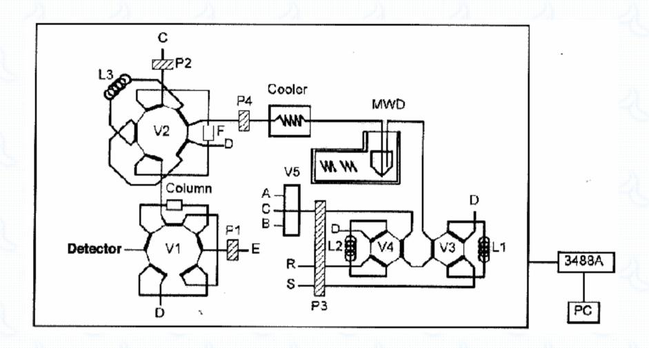
P1 and P2: pump with set flow, P3 and P4: pump with continous flow
