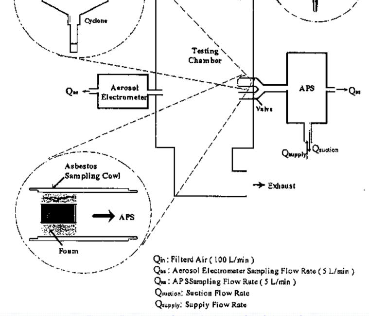
Figure 7 Experimental System for Aerosol Size Selective Sampler
