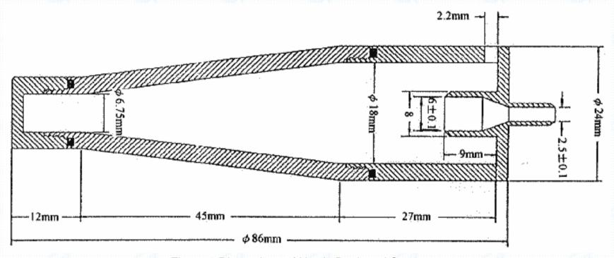
Figure 6 Dimensions of Newly Designed Separator
