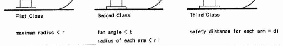
Figure 5 Safety Protection for Robots: Classification and Parameters
