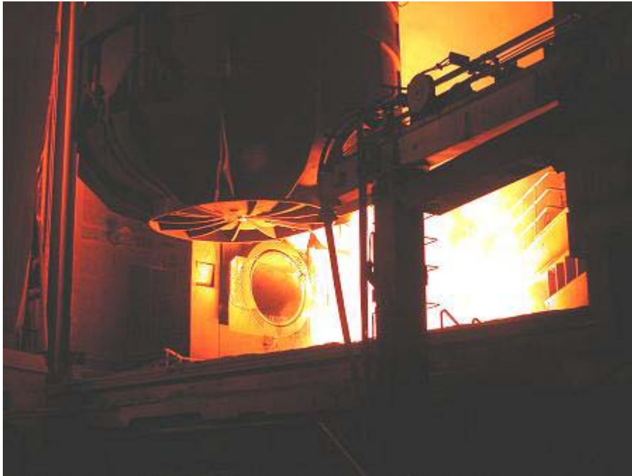
Figure 7 Smelt process using electric arc furnace in ferrous metal refining plant-feeding
