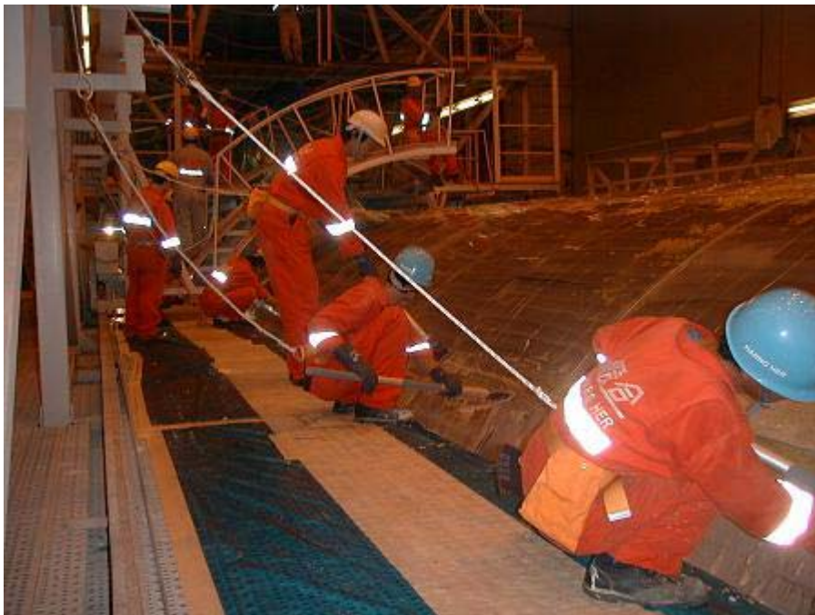
Figure 6 Paint stripping work during aircraft maintenance
