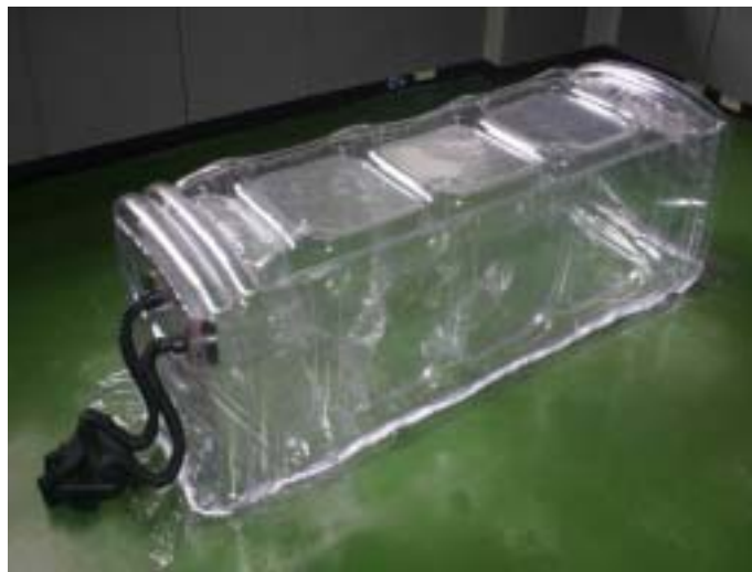
Figure 6 Mobile negative mobile pressure isolation chamber
