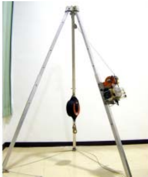
Figure 4 Falling prevention and emergency aid tripod hoist
