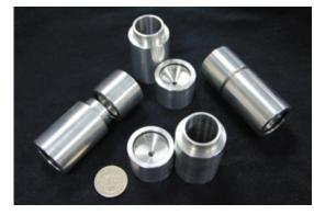
The appearance and size of the uniform aerosol deposit sampling device (compared with a NTD\$10 coin)
