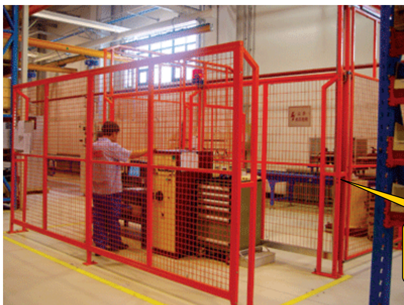
Illustration 2.2 Installation of protection and isolation devices.
