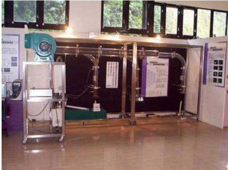
Fig.6 Local ventilation training equipment with variable wind flow adjustment
