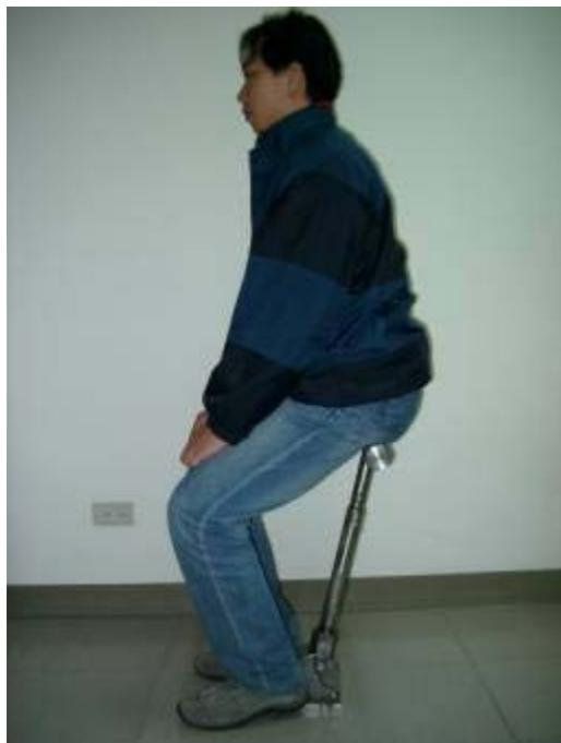
Fig.7 Sit-stand dual purpose chair for use in semiconductor clean room
