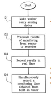
a flowchart of a method of monitoring the exposure levels of workers according to preferred embodiment of the invention.
