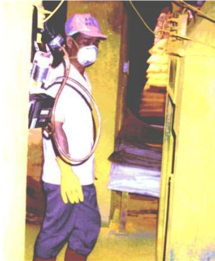
Figure 5: Determination of particle size in bagging chromic lead
